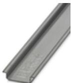
DIN rail, unperforated, Standard profile, width: 35 mm, height: 7.5 mm, acc. to EN 60715, material: Stainless steel V2A, uncoated, length: 2000 mm, color: silver
